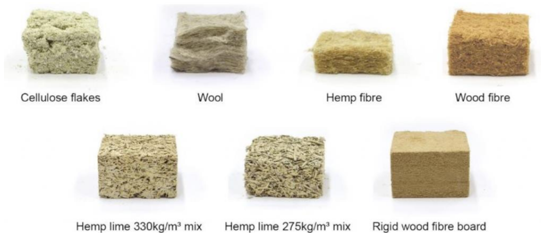
Figure 2-2 Example of bio-based insulation materials.
